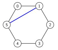
To induce the complete graph on  $\{0,1,2\}$ : Local complementation on 1. To induce the empty graph on  $\{0,1,2\}$ : Local complementation on 0,
